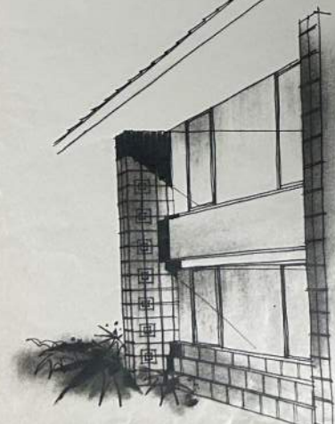
CONCRETE BLOCK COLUMN FOR TWO STORY STRUCTURES SPACING APPROX. 12'-0"
